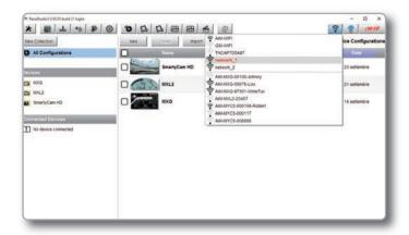
Once the user's PC is authenticated to the same network called "network\_2," it can see the AiM device previously configured to gain access to the target network.
