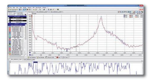
20 samples per second let you have a cleaner signal, and make easier to see the RPM trend, while 50 samples per second let you better recognize the vibration of the chassis and all the strengths that can create problems to the ideal movement of your kart.
