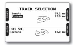
The tracks in the dbase are shown in the upper part of the display. The nearest are shown first. You will see the name of the track, the shape, and the distance from where you are. In the lower part of the track, the selected track is shown.
