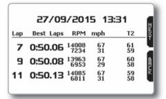
It shows the best three laps of your test, giving the information about maximum and minimum RPM, speed, and temperature(s) for them.
