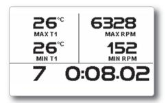
■ In Oval racing MyChron5 shows: Lap Time and RPM drop ( difference between max and min RPM)
